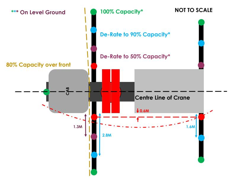
The stabilisers can be extended individually (do not have to be extended equally), the Fassi Computer will calculate the duty when lifting directly over each leg in sectors.
